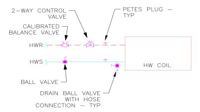
1) It is allowed to use a combination valve assembly such as the Flow Design Inc. model UA or UB with included NPT union connections and optional pressure/temperature ports, and manual air vent on the return water side. Model UA or UB with included NPT union connections and optional pressure/temperature ports, and hose end drain on the supply water side. Approval by Owner is required prior to installation. b. Supplemental AC unit/heat pump piping:
